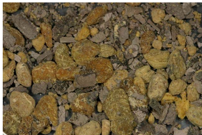
Mud and pollen from track around window in home (PES 2008).
